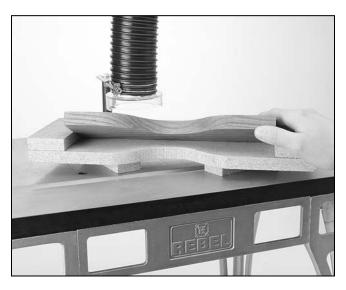
Figure 24. Inverted Fixture with workpiece.
